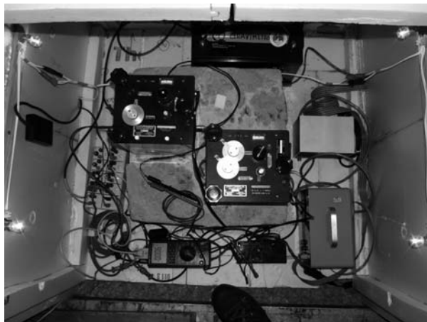
Figure 7: Set-up of the instruments at a grounded pillar within the gravimetry hut, Belgrano II: IAA gravity meter L&R G-748 (left), TUD gravity meter L&R D-193 (right).
