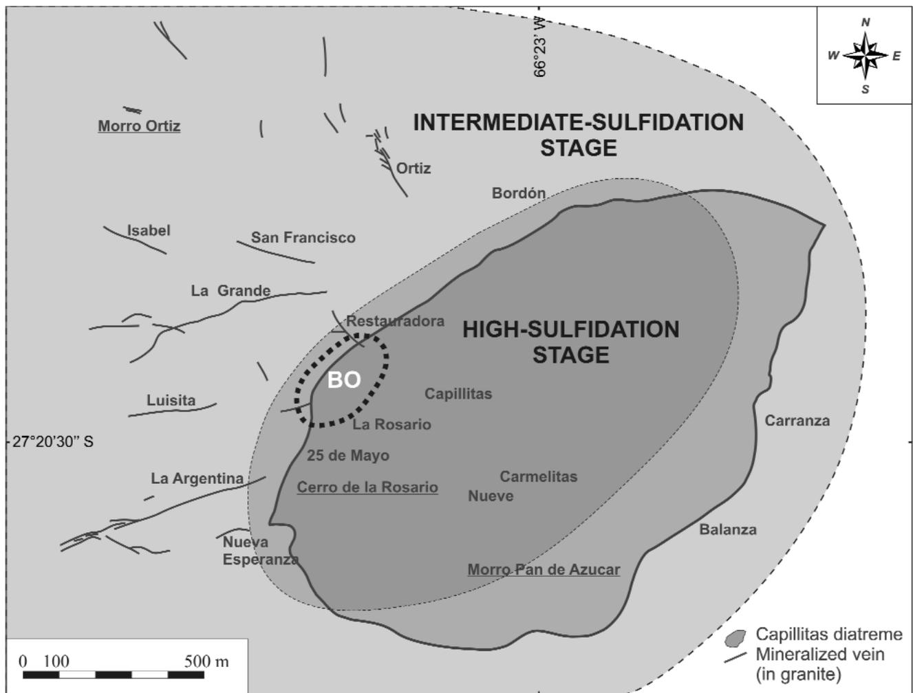
**Figure 1:** Simplified geologic map and estimated zonation of the epithermal mineralization at the Capillitas deposit. The high-sulfidation stage mineralization was overprinted by the intermediate-sulfidation stage mineralization; BO = bornite-chalcocite-digenite-rich ores.
