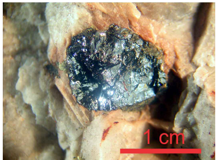
Figure 2. Photograph of one dark grey cm-sized prismatic crystal of niobian rutile with the [001] axis approximately normal to the surface of the sample, included in plagioclase in the core-margin association of the Rancul pegmatite. Note the oxidation halo around the crystal.
