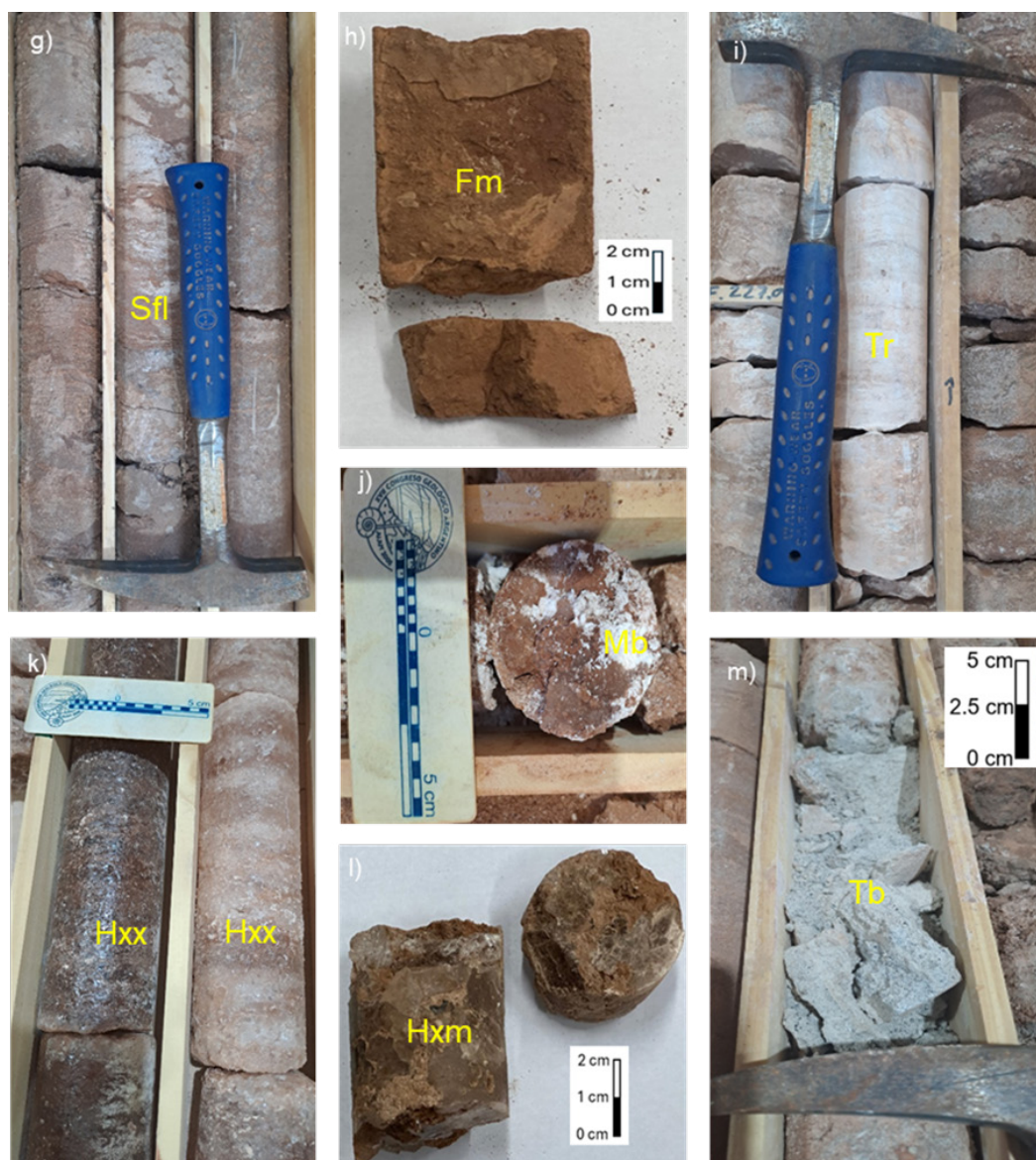
Figure 5. Core sample showing various facies. g) Sandstone facies with flaser structures (Sfl), thin pelitic laminae (brown) can be distinguished within the sandy matrix (whitish), h) Core fragment with pelitic facies (Fm), the fracture shows a massive structure and absence of lamination, i) Travertine facies (Tr), is observed the whitish color with well-defined parallel lamination, j) Disintegrated Mb facies, represented by white crystals and silky luster in Fm facies, k) Crystalline halite facies (Hxx), displaying a pink and brown color with massive structure, l) Fragments of muddy halite facies (Hxm), is observed the pelitic matrix, m) Sample of disintegrated volcanic material (Tb).
