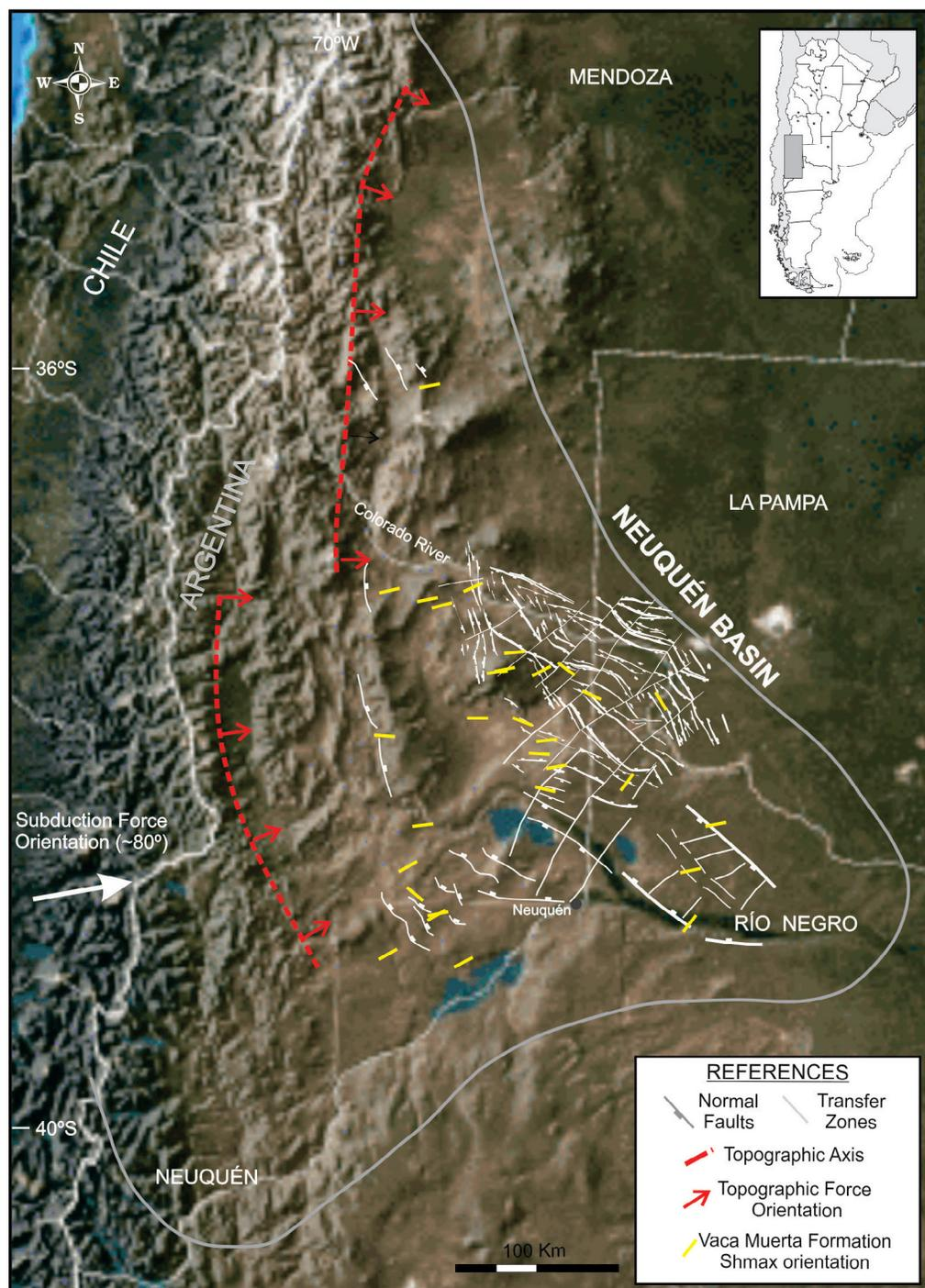
**Figure 1:** Maximum horizontal stress (SHmax) distribution, orientation for 30 wells distributed along the Neuquén Basin for the Vaca Muerta Formation. The main forces and controls acting over the horizontal stress field for the Vaca Muerta Formation are also shown: the subduction force, the topographic axis and the Upper Triassic - Lower Jurassic grabens (Cristallini et al. 2006, Bechis et al. 2014).
