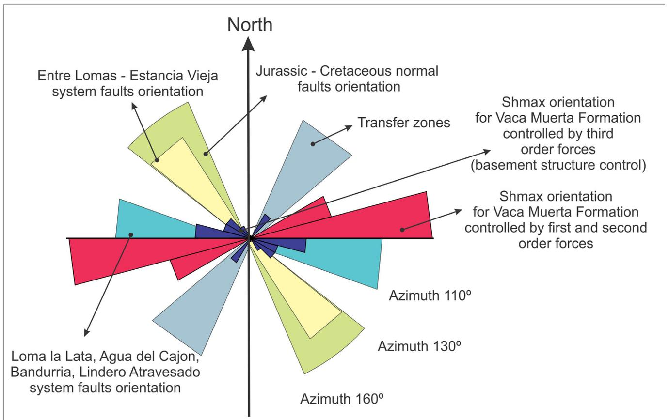
**Figure 4:** SHmax orientation obtained for the Vaca Muerta Formation plotted with the system faults as proposed by Cristallini et al. (2009). It can be seen that the SHmax orientations not controlled by subduction or topographic forces are controlled by the differential subsidence of the grabens and half-grabens infill or transfer zones.
