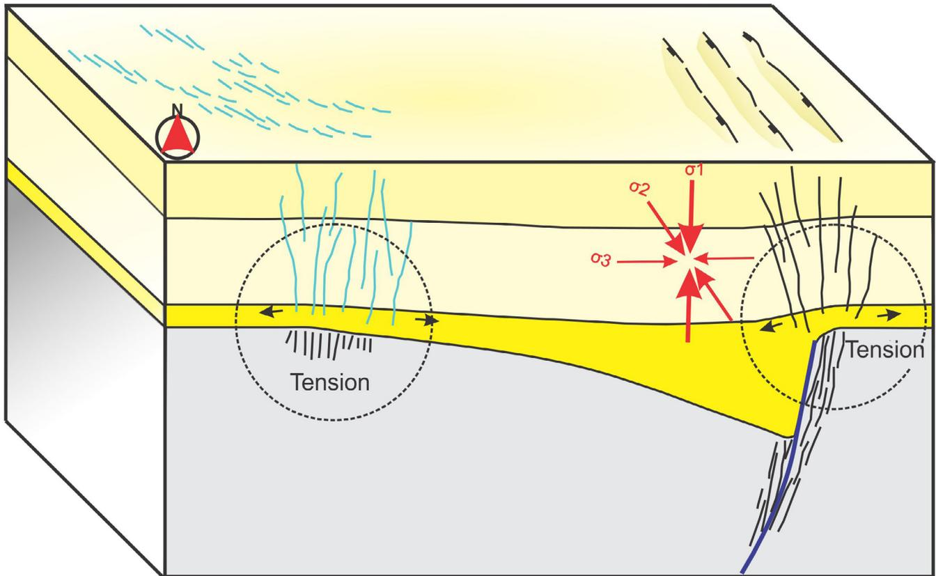
**Figure 3:** Normal faults developed as a result of the tension associated with differential subsidence (modified from Cristallini et al. 2009).
