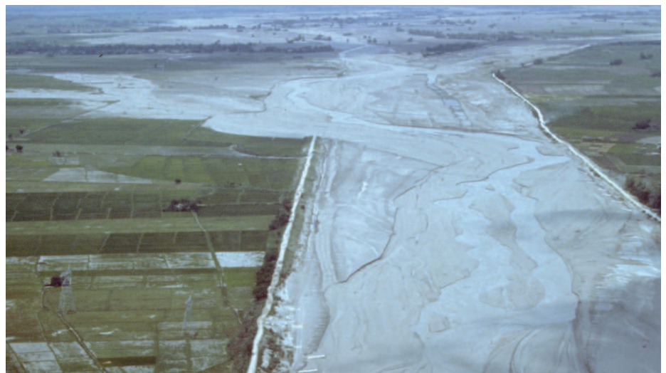
Figure 6. The valley of Bamban River in the Philippines following the eruption of Mount Pinatubo in 1991. The floodplain was buried in lahar and fluviially resedimented ash deposits eroded from the flank of the volcano. The protective river dykes have been breached and alluvial sediments spread over farmland and villages. (Photo by Willie Scott, courtesy of U.S. Geological Survey.)
