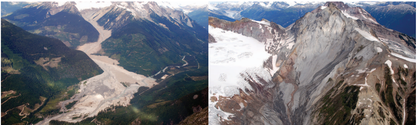
Figure 4. Source area and path of the 2010 Capricorn Creek landslide (ca. 40 \times 10^6 \text{ m}^3 ) in the southern Coast Mountains of British Columbia. The landslide occurred in warm weather in thawing, highly fractured volcanic rocks.
