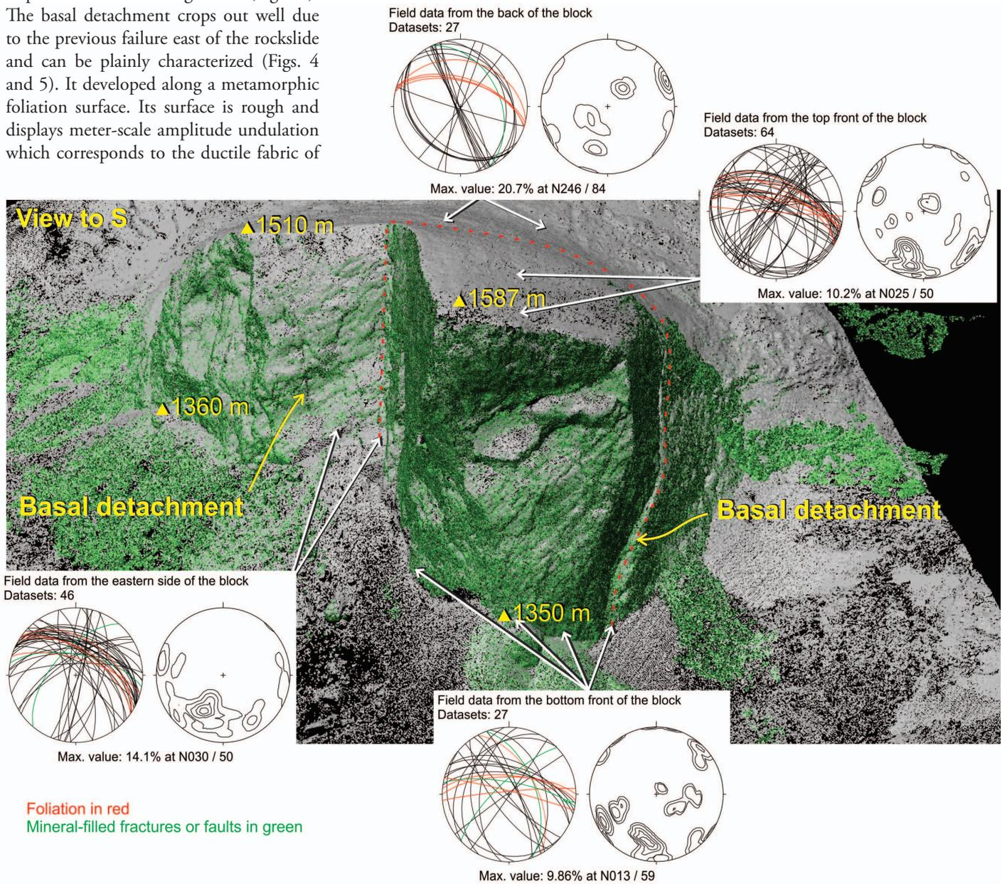
**Figure 4.** Stereoplot of structural field measurements at locations shown on a 3D view of Svarttinden. The green dots are the TLS point cloud superimposed on the hill-shaded ALS-DEM in gray; the red dashed line is the trace of the single basal detachment of the translational rockslide.
