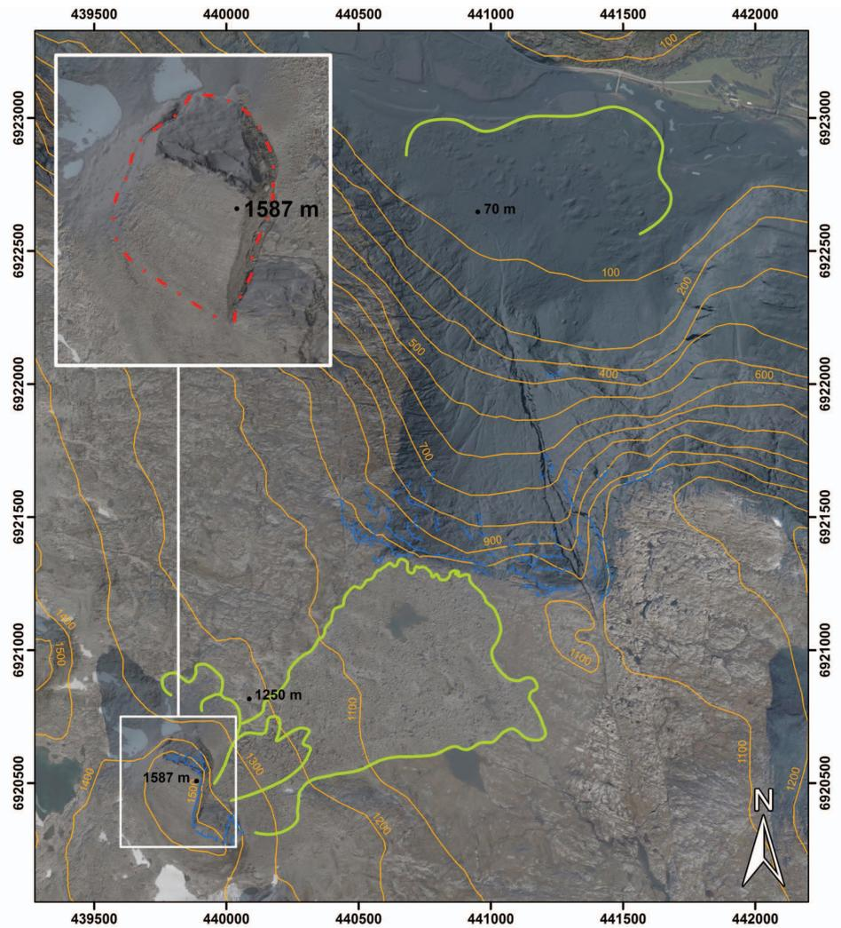
**Figure 3.** Svarttinden: a large remaining rock slope instability west of a previous failed slope (in white frame). Blue lines: scars of previous rock slope failures; green lines: limits of deposits of previous failures; red dashed line: trace of the single basal detachment of the translational rockslide.
