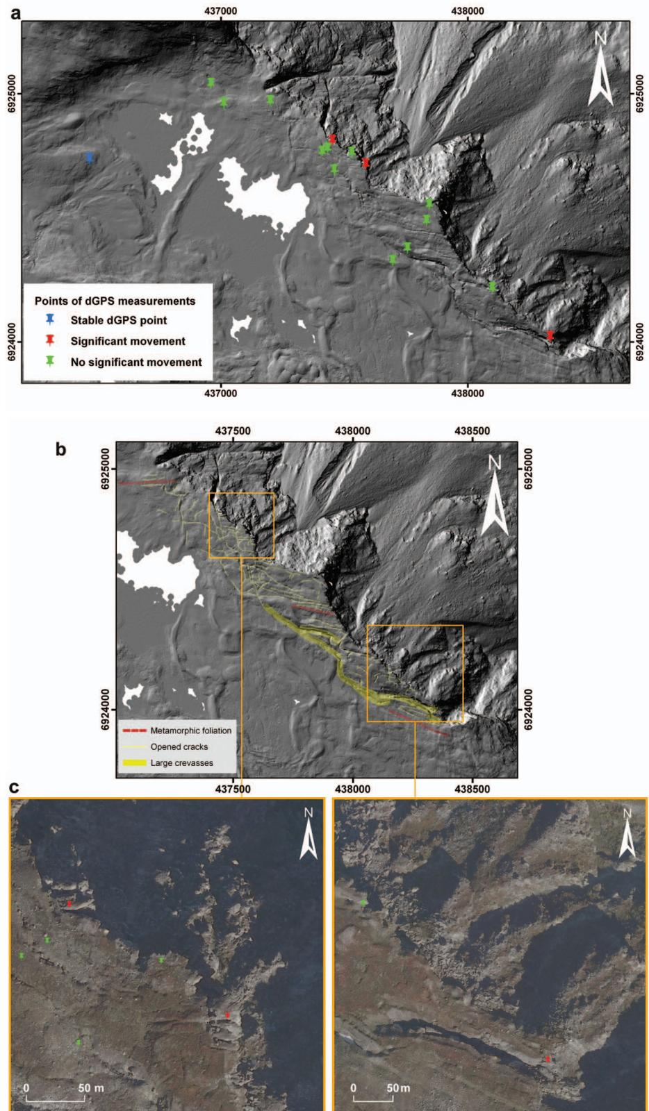
**Figure 12.** a) Hillshaded ALS-DEM of the Børa plateau with dGPS antenna positions and associated detection of movements. The movements are significant on 3 local instabilities at the edge of Børa plateau and range between 0.2 and 2 cm/yr. b) Structural map of the deformed edge of Børa plateau from the analysis of the ALS-DEM. c) And d) detailed aerial photographs of the three local instabilities.
