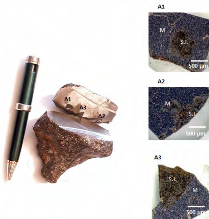
Figure 1. The San Juan A mass and a view of the slide where the three silicate inclusions (A1, A2 and A3) are seen. A detail of the three polished sections A1, A2 and A3 are shown. M: Metal; S.I.: Silicate Inclusion.
