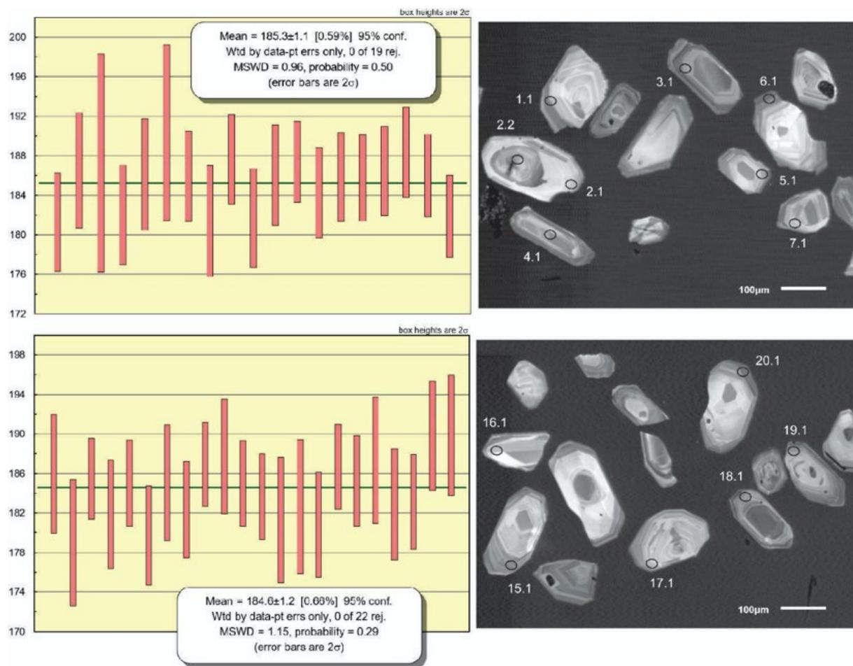
**Figure 2.** SHRIMP U-Pb zircon ages of two samples of the Cabo Blanco. Left: Relative probability plot of U/Pb zircon ages. Right: cathodoluminescence images of dated zircons (black circles and numbers mark microprobe shots).
