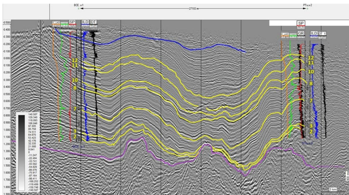
**Figure 1.** Seismic section from BCE x-1 to PTu x-2 wells. Correlation lines (yellow) correspond to the event number (#) in Table 1. The purple line corresponds to the top of the Precuyano; the blue line indicates the base of the Vaca Muerta Formation. Abbreviations: C-LAD: cumulative last appearance datum in the drilling direction; RICHNESS: specific richness; DT: sonic profile; ILD: deep resistivity; GR: gamma ray; SP: spontaneous potential.
